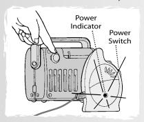
Place transmitter in room in which you intend to use it. Rotate transmitter power switch to turn power on. Power indicator lights. Turn on a radio.
